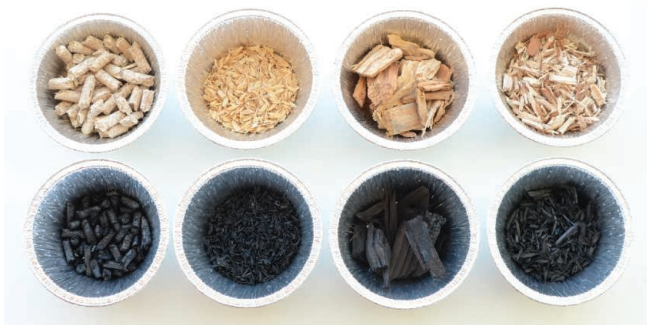
Biochar variation. The diverse properties of biochar have led to widely varying results. A more systematic understanding is now emerging, helping to define its value in crop production and carbon storage.
