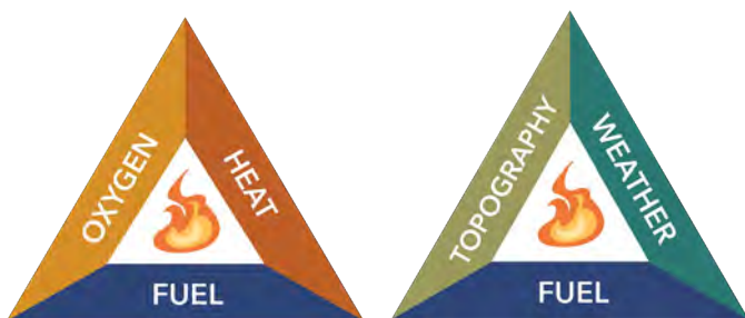
Figure 8.1. The fire triangle (left) & fire behavior triangle (right). These show the ingredients of fire & the 3 environmental factors that affect fire behavior. Fuel is the only one of these five factors that can be manipulated. Fuels management is a primary objective in firescaping.
