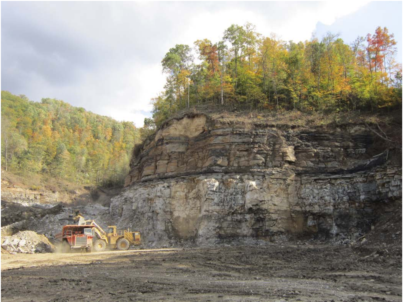
Fig. 1. Example of a stratigraphic profile of geologic materials disturbed by an Appalachian surface mine operating in previously unmined terrain. The uppermost materials are soils and vary in thickness between 0.3 and 1 m. The rock materials immediately below the soils to a depth of approximately 10 m are brownish in color because they have been affected by surface environmental processes, and are said to be “weathered.” Below the weathered rocks are lighter-colored rock materials, often said to be “unweathered.”
